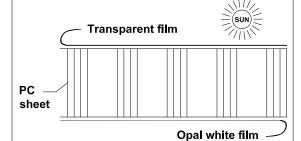
Two sides of PC sheet are covered with thin film, one side's film is transparent, another side's film is opal white. The UV-protected side of PC sheet is covered with transparent
