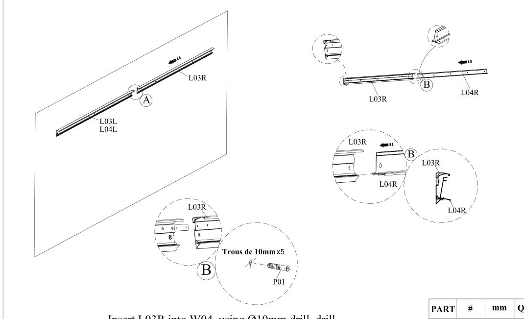
Insert L03R into W04, using Ø10mm drill, drill 5 holes on the wall located by the holes on L03R, then take L03R, put P01 into the holes.
