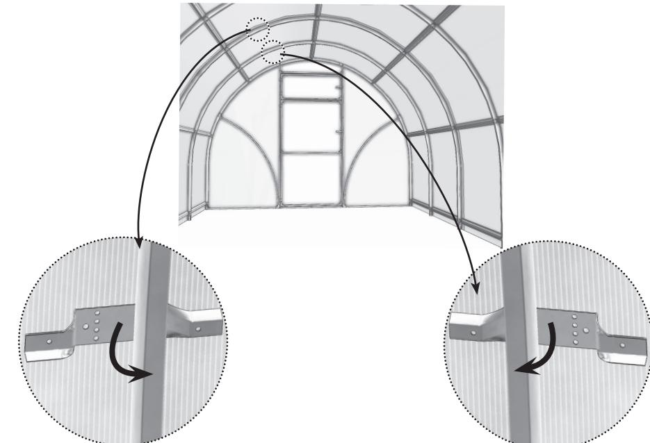
Kinnitage surukid isepuurivate kruvide abil. Paigaldage surukitesse latt **C.02**.
